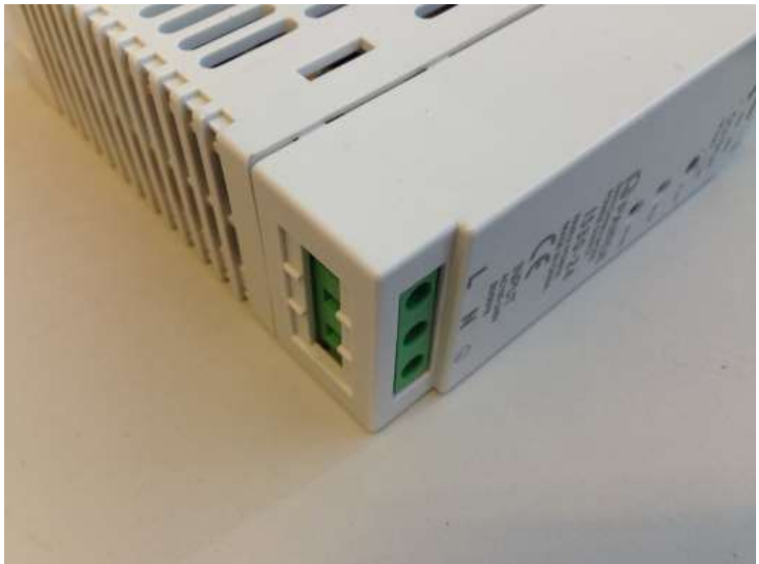
FIGURE 10. SWITCHING MODE POWER SUPPLY (M/N: IS30-24) AC IN
